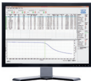
PC control for representative results OXITEST is controlled via PC; tests are performed directly on the whole sample without the need for preliminary fat separation.
