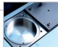
Two separate titanium chambers in order to test the same sample in duplicate or different samples at the same time.
